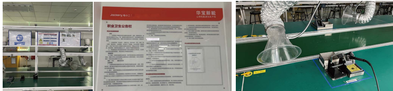
Display notification cards for positions exposed to occupational hazards, standardize labels for wearing protective equipment and distribute protective supplies, including masks and gloves, on a daily basis
